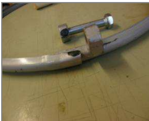
Fig 1 – A clamping band with a failed spot weld (nut detached)
