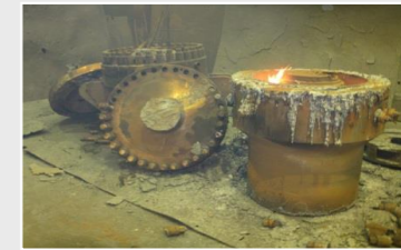
Primary Circuit Circulator from Winfrith being size reduced
