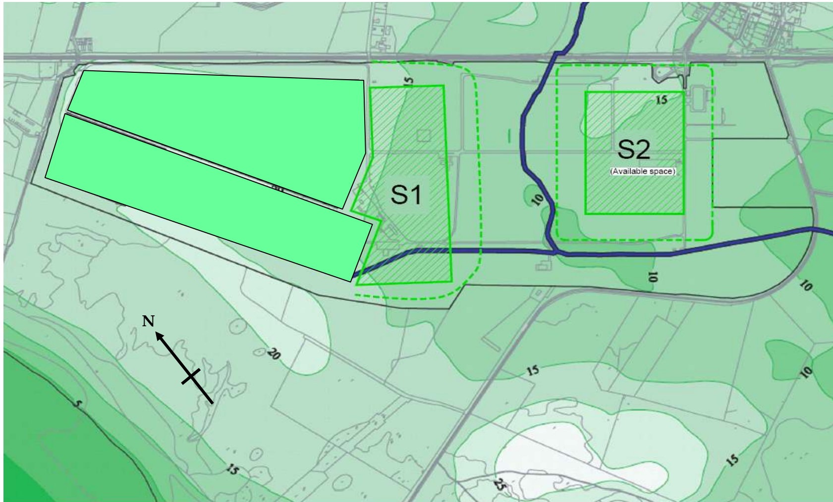
Figure 2: Map of the LLWR, showing the licensed site boundary and topography (after BNFL, 2002; original reproduced from the Ordnance Survey map by permission of the Ordnance Survey), with the potential locations and geometries for additional vaults marked as S1 and S2. Geometries correspond to that required for Inventory Case A, except for S2, for which the footprint is allowed to be constrained by site features.
