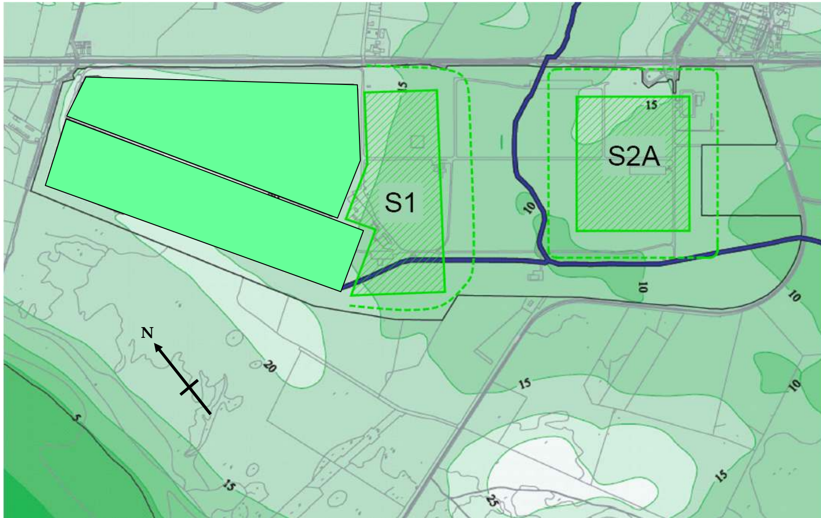
Figure 3: As for Figure 2, except that S2 dimensions are increased to indicate required footprint to accommodate all Case A inventory wastes
