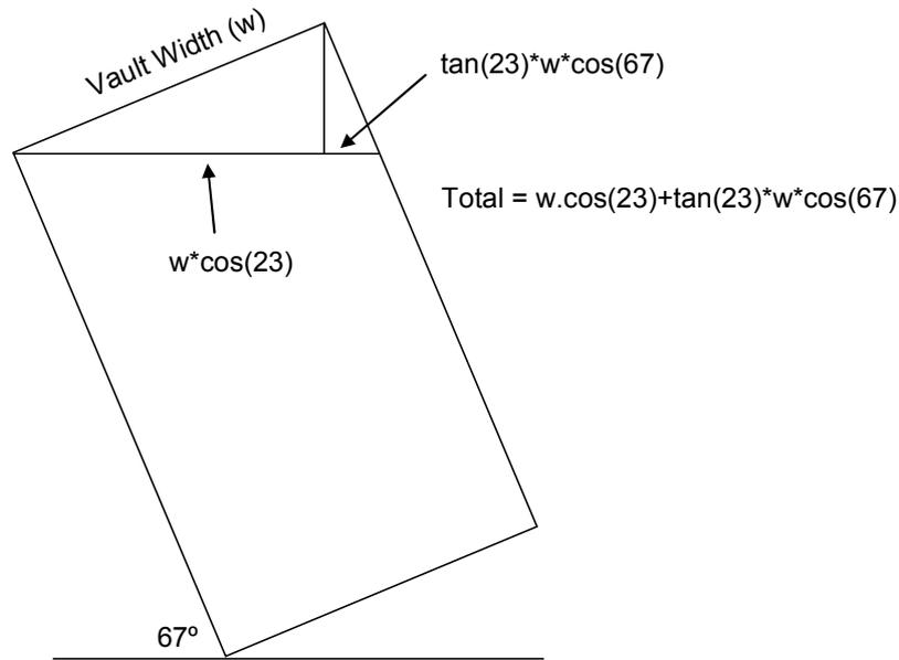
**Figure 4-1. Calculation of the vault length exposed in the cliff**
