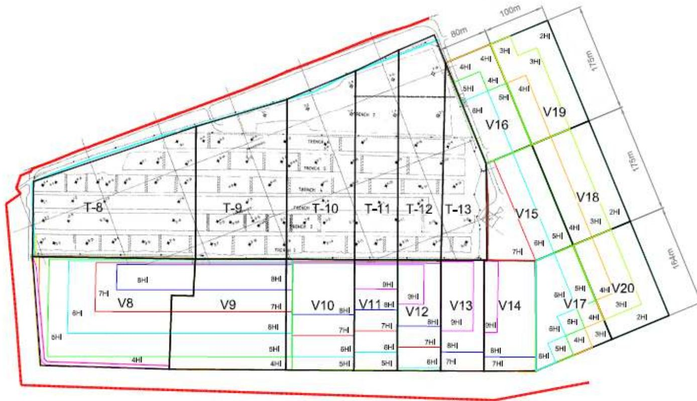
Figure 2-1: Layout of the extended facility, showing the six additional vaults (Vaults 15 to 20)
