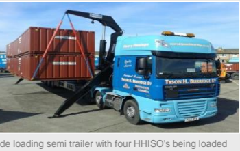
Side loading semi trailer with four HHSOs being loaded
